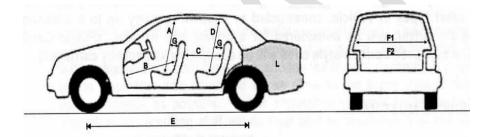
93cm/36" min. Α Cushion not compressed. В 96cm/37" min. Seat fully rearwards. C 61cm/41" min. Front seat fully rearwards. D 84cm/33" min. Cushion not compressed. Ε Wheelbase 245cm/96" min. F1 133cm/52" min. Interior width between doors F2 122cm/48" Between armrests
